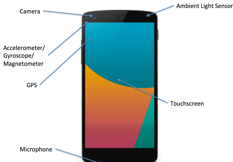
Figure-2: Position of Sensors
